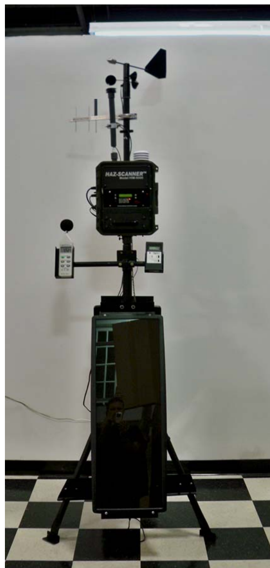
HIM-6000 Shown with optional tripod stand & solar panels Atomic Radiation and Noise level Meter
